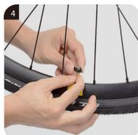
4. With the tire deflated, use the Giant Valve Core Remover to unscrew and remove the core from the valve, and then add sealant through the valve.
