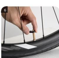
6. After adding sealant, re-install the tubeless valve core using the Giant Valve Core Remover. Ensure the valve core is firmly seated within the valve.
