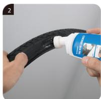
2. Apply Giant Tubeless Tire Lube on the tire bead and the area where the ERT liner meets with the tire. This not only makes tire installation easier, it helps the tire seat more uniformly during inflation.
