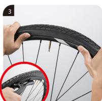
3. To install the tire, first insert the valve through the valve hole on the rim. Then, begin installing the tire from the opposite side of the rim from the valve, working your way around the rim and back toward the valve. Once the tire is fully seated on the rim, ensure that the tire beads are resting in the rim's center channel.
