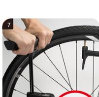
7. With the valve core installed and in the open position, inflate the tire to the maximum pressure indicated on the tire's side wall. This step is necessary to let the sealant distribute evenly inside the tire. Make sure the safety line on the sidewall of the tire is visible all the way around the rim, on both sides.
