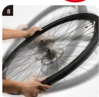
8. If the safety line is visible all the way around the rim on both sides, rotate or shake the wheel to spread the sealant throughout the tire to fill any small holes in the casing that could allow air to escape.
